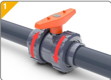
**1.** Remove the valve body from the installation. Loosen the nuts according to the arrows.
